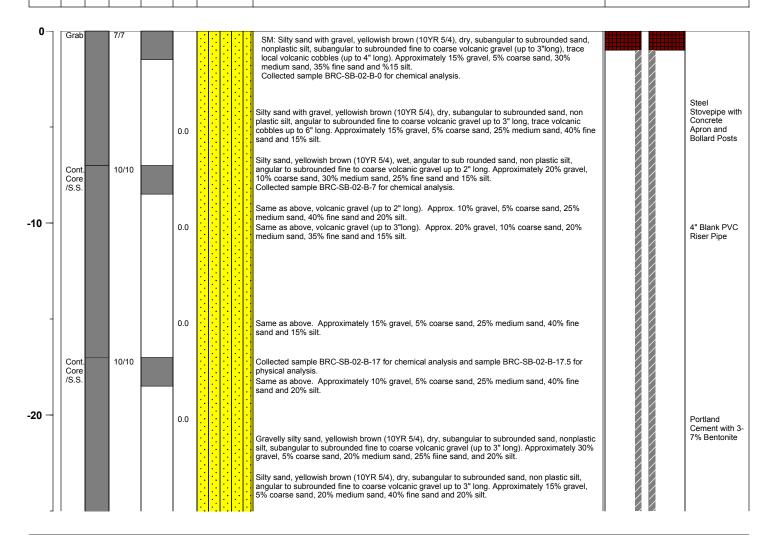
Project No. 3850360 Log of Boring: BRC-SB-02-B
