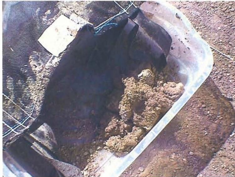
**Figure 4-8. Material from TIMET pond SW-2 after one week of dewatering, September 2004.**
