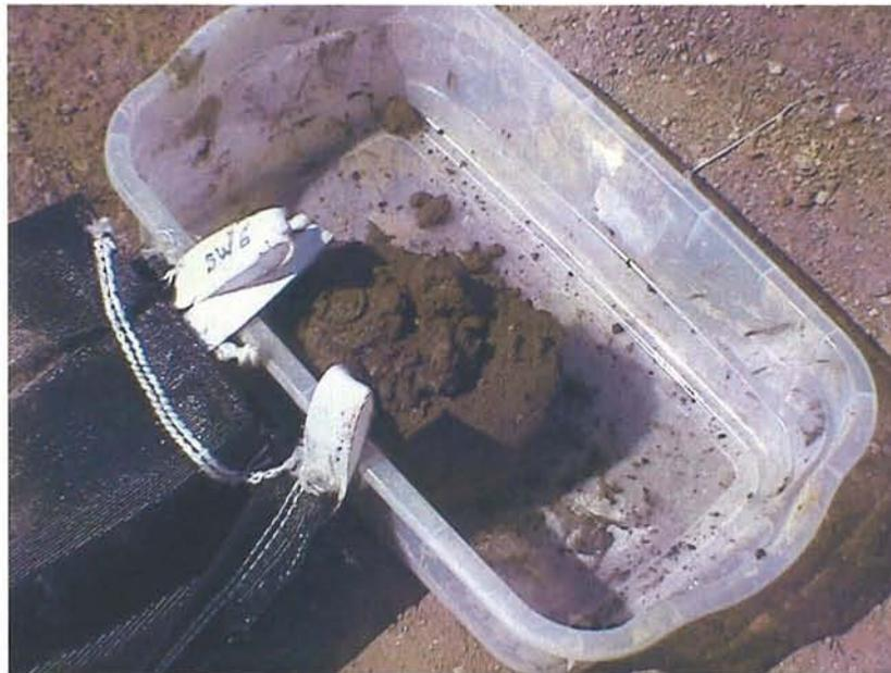
Figure 4-12. Material from TIMET pond SW-6 after one week of dewatering, September 2004.
