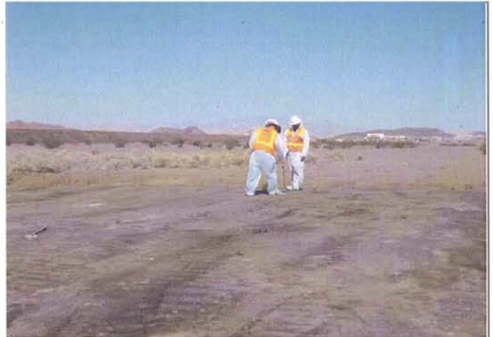
Eastside, Geosyntec performing compaction testing on test pads..
