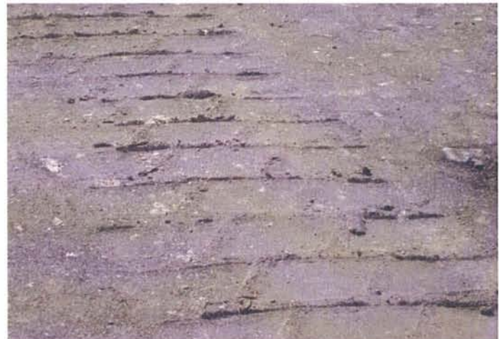
Eastside: Rutting was minor after 40 ton loaded dump truck backed on test pad.
