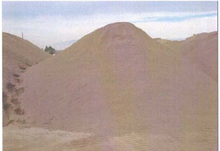
Eastside: WST-1, Powerscreened 1" minus, soils. Inspected by Weston.
