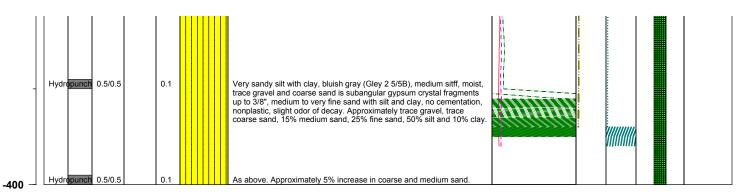
Project No. 3850360 Log of Boring: BRC-SB-12-A
