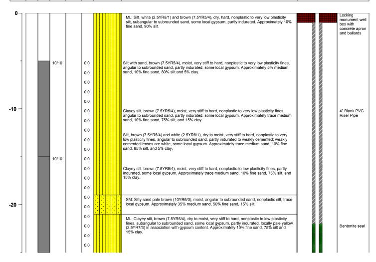
Project No. 3850360 Log of Boring: BRC-SB-07-B
