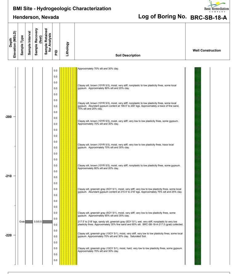
Log of Boring: BRC-SB-18-A
