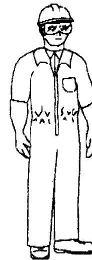
LEVEL D Protection Basic work uniform, i.e. longsleeve coveralls, gloves, hardhat, boot, faceshield or goggles.
