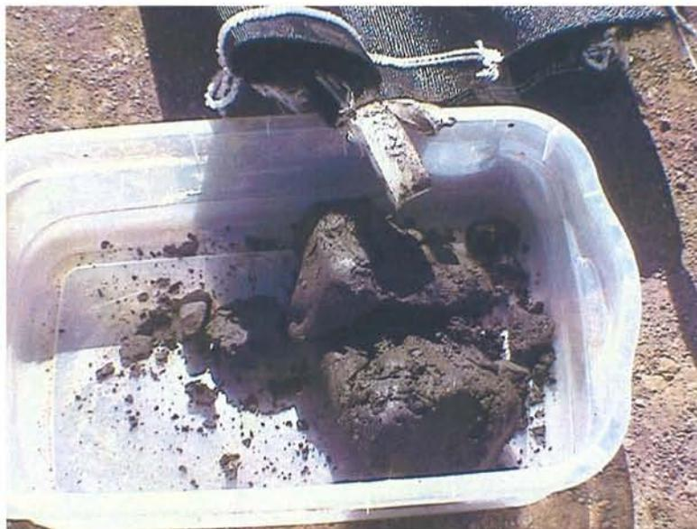
**Figure 4-5. Material from TIMET pond SW-11 after one week of dewatering, September 2004.**
