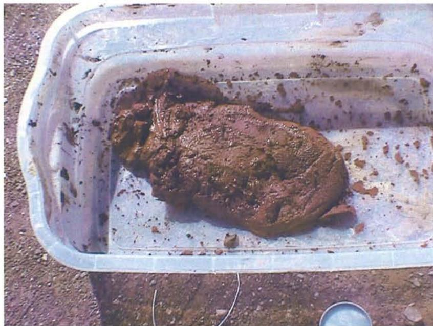
**Figure 4-10. Material from TIMET pond SW-12 after one week of dewatering, September 2004.**
