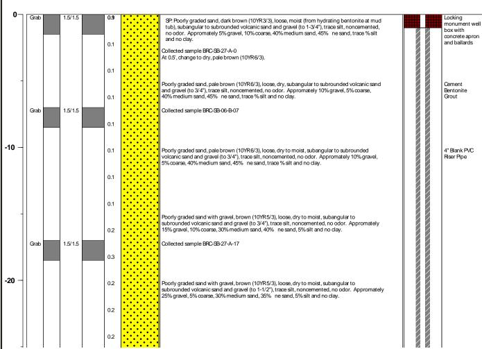
Drilling Method:Rotary SonicBorehole Total Depth:400 ft bgsDrilling Equipment:Rotary SonicBorehole Diameter:8.5"
