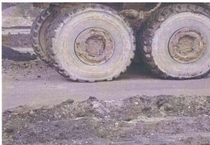
Eastside: Loaded haul truck on test pad, checking for deflection.
