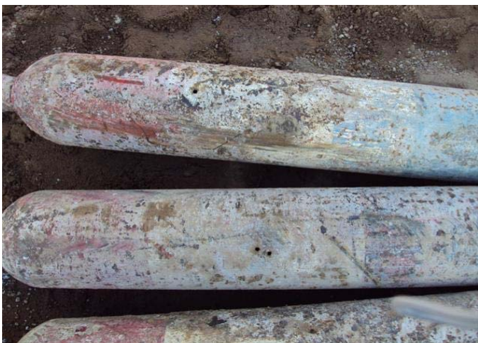
CAMU: Cylinder/bottles from slit trenches, previously drilled holes.
